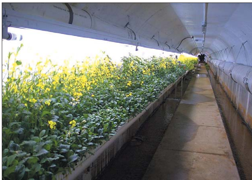
Figure 5. Transgenic Brassica juncea (Indian mustard) grown in a contained hydroponic setup (a mine drainage tunnel in Leadville, CO) to test the altered plants' capacity to remove metals from polluted water.
